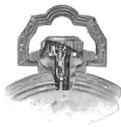
Cross Section Illustrating Construction of Pendant and Crown
