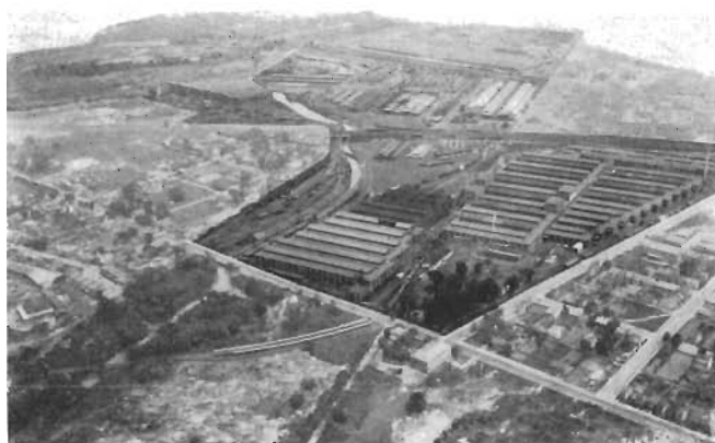
Aeroplane view of the Baldwin Locomotive Works (at left), Eddystone Plant on the Delaware River, fourteen miles below Philadelphia, where the Frisco's new engines were built. The water front has a dredged channel to accommodate the largest vessels and crane facilities for loading complete locomotives from the tracks to ships.
