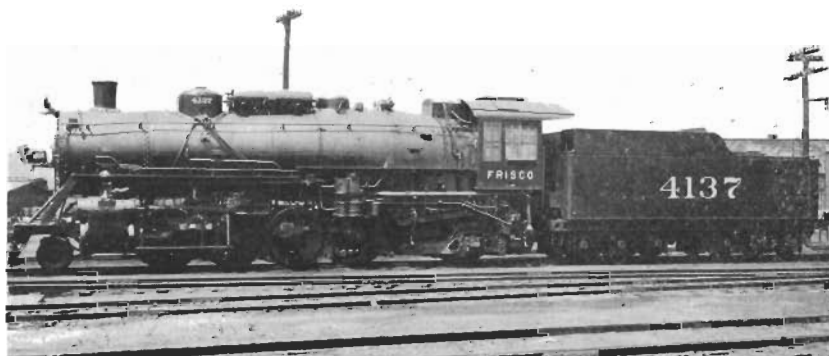
The Mikado type freight engine, shown above, is one of the fifteen of its kind delivered to the Frisco last month. It embodies the latest locomotive improvement, and was constructed by the Baldwin Locomotive Works at its Eddystone plant.
