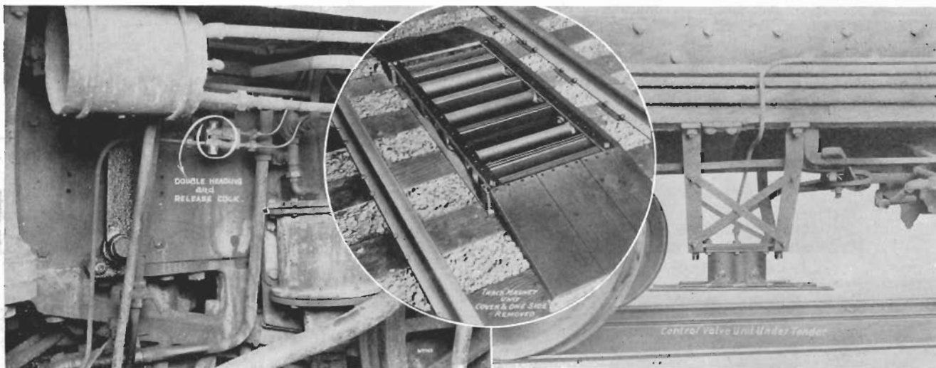
At the left in the above picture, in white circle, is the double heading and release cock, under the engine. The circular insert shows the track magnet with cover and one side removed, and the picture at the right shows the position of the control valve unit under the tender
