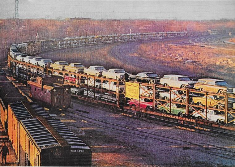
The St. Louis-San Francisco Railway, pioneer in this modern method of transporting new automobiles, has conducted exhaustive tests to assure clean, damage-free shipment.
